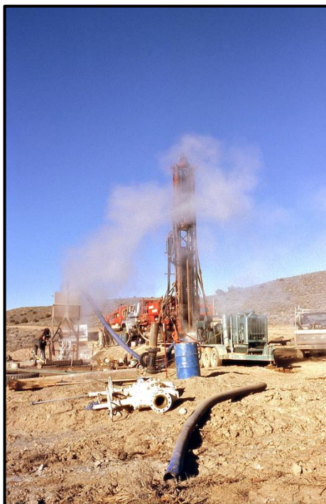
A Gypsy drill hole. Picture taken on a cold day with mist rising off the warmer drilling mud tank.
