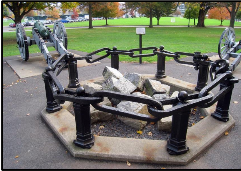
Fig. 7. A section of the Great Chain that stretched across the Hudson River at West Point. Each link is about 2 feet long and as big around as a man's arm. To break through the chain, the British would have had to expose their ships under the surrounding cannon batteries while trying to cut through the chain. All the while they would also have to deal with the river's swift current, tides, and shifting winds. The British never tried to surmount this geomorphic and man-made defense.
