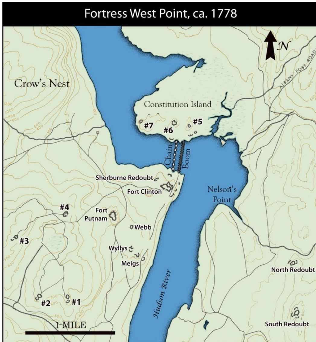
Fig. 6. Kosciuszko's fortification of the Hudson River at West Point includes the main battery at Fort Clinton and a series of batteries and redoubts on Constitution Island and at high points along both sides of the river.
