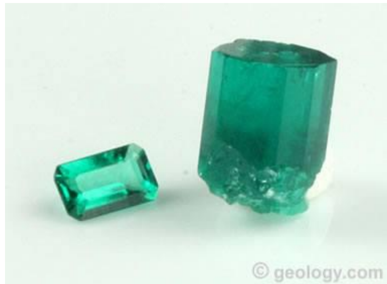
Synthetic emerald: The materials in this photo are lab-created or synthetic emerald produced by Chatham. On the left is a faceted synthetic emerald weighing 0.23 carats and measuring
